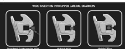
Compared to standard rectangular wire, the shape of SmartClip™ Hybrid Rectangular Archwire provides more tolerance in the wire alignment to the bracket slot without encountering a contact point interference (arrows).
